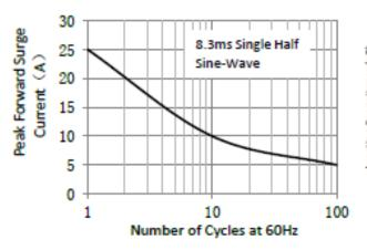
Figure 5. Maximum Non-Repetitive Peak Forward Surge Current
